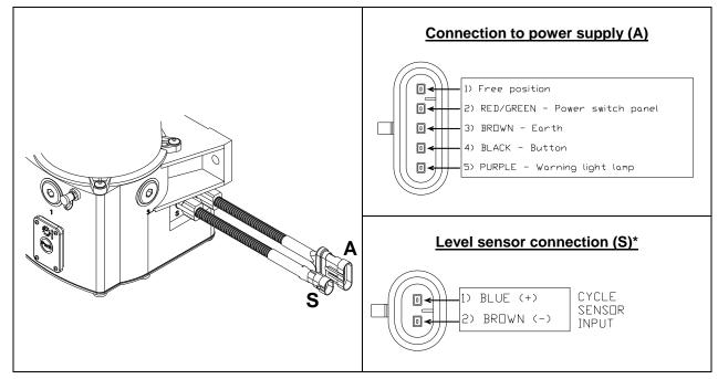
\* Note: Compatibility is guarantee only with microswitch and REED contacts. Pause-sensor timer doesn't work with proximity switch.
