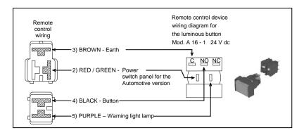
To connect the Remote Control device to the electro-pump, please refer to the electric diagram of the pump you bought.
