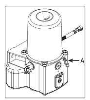
Reservoir is refilled through lubricator "A". Remove the lubricator plug and refill the reservoir up to maximum level (MAX), by means of a special equipment for lubrication in pressure. During refill, verify that air is discharged through the air-hole. Ensure that the air-hole, placed on the reservoir rear side, is not obstructed.
