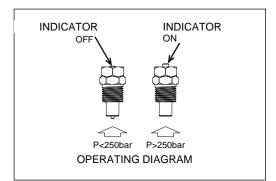
During ordinary operating conditions, the external overpressure indicator is at rest (**OFF**). As soon as pumping element outlet pressure reaches 250 bar (3675 psi), the indicator moves to signalling position (**ON**). After the restore of ordinary operating conditions, it is necessary to verify that the over-pressure indicator is in the **OFF** position.
