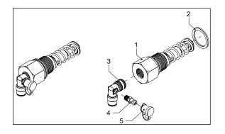
The aside figure shows a pumping element with the fitting for the main pipe connection, which is supplied as standard. The main components are:
