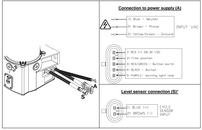
\* Note: Compatibility is guarantee only with microswitch and REED contacts. Pause-sensor timer doesn't work with proximity switch.
