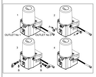
The system is usually supplied with a single pumping element installed on outlet 2.
