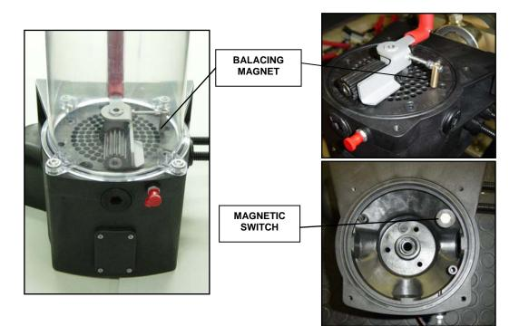
The **magnetic switch** operation is based on the principle of *normally open switch*. When pump is switched on, the grease scraper drags the **balancing magnet**. At this time, one of the following conditions can be generate:
