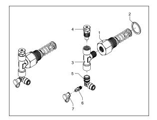
The pumping element can be supplied, as optional, with an indicator which includes an external signalling device controlling safety valve operation. The following table lists the components:
